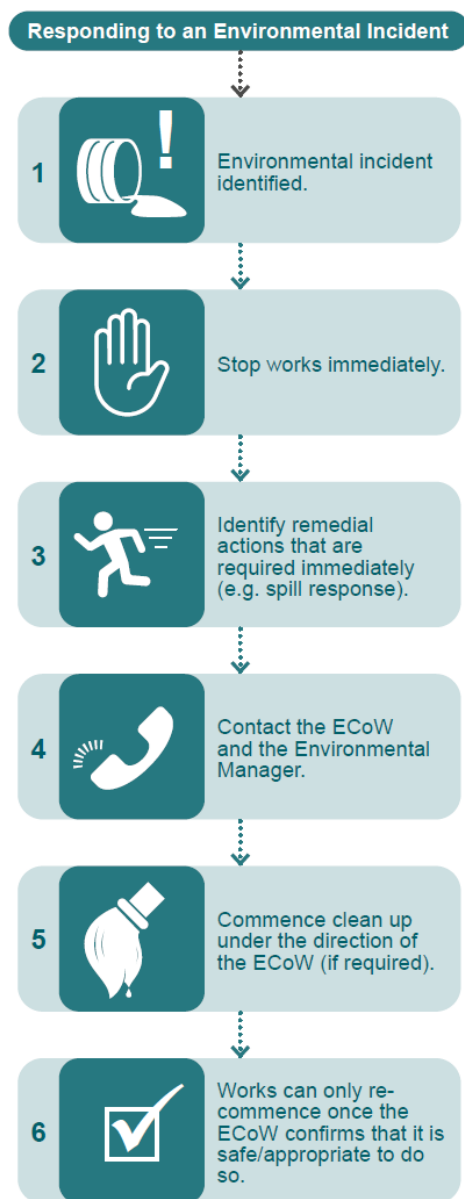
Figure R.1: Environmental Incident Response Process
